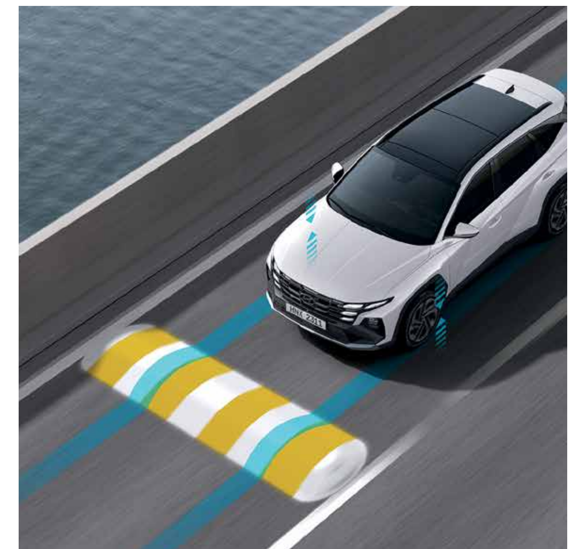
e-Comfort Drive When passing speed bumps, the hybrid technology helps reduce vehicle shaking (pitch motion), resulting in a smooth ride even on uneven roads.
